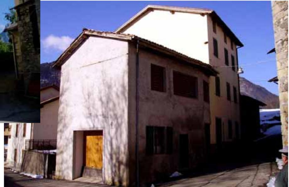
Comune di Paluzza (UD) 3297 GG –  $S_{Netta}=355$  mq –  $S/V=0,61$  –  $PT_{Risc}=11,8$  KW –  $IE=43$  kWh/m<sup>2</sup>a
