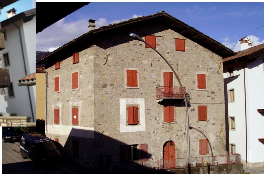
Comune di Sutrio (UD) 3487 GG –  $S_{Netta}=370$  mq –  $S/V=0,60$  –  $PT_{Risc}=9,1$  KW –  $IE=34$  kWh/m<sup>2</sup>a
